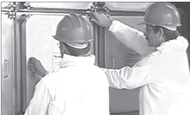
Alternate tightening knobs for best door seal.
