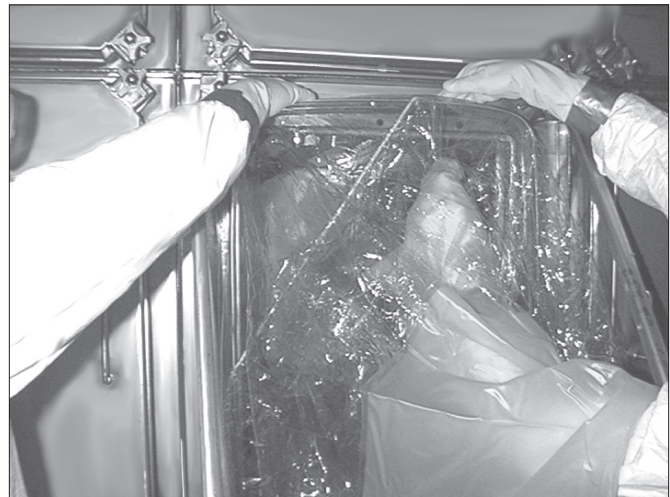
Remove old bag stub using new bag glove sleeve.
