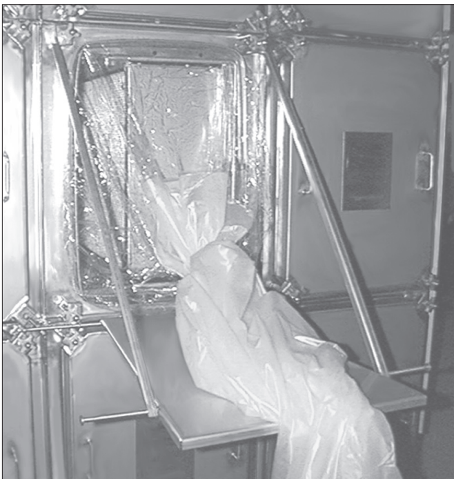
Extend bag and inspect carefully to ensure that the bag has incurred no damage.
