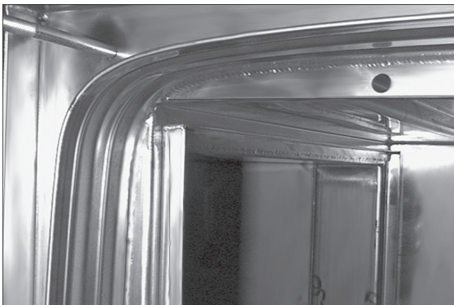
Housing knife edge front and top.
