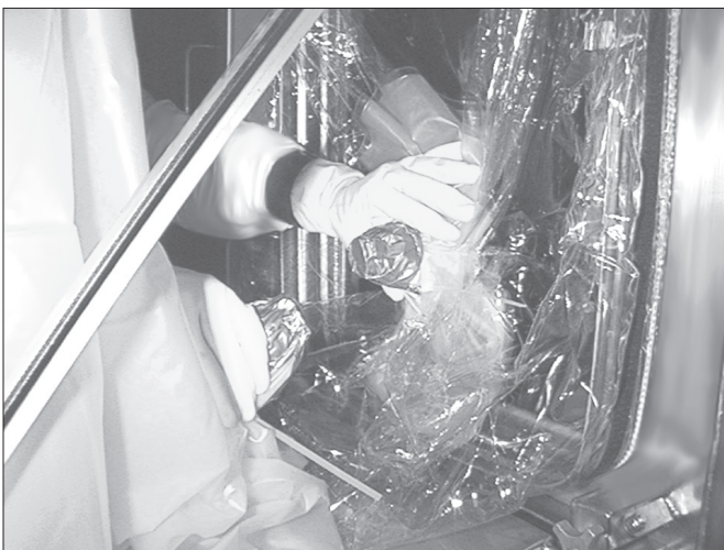
Place tape over cut bag end.
