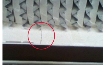
Figure 3: Photograph of a stress crack in filter design A
